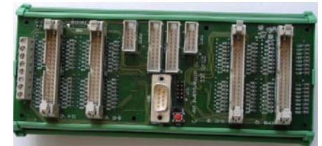
General-purpose plug-on I/O module for the monitoring and control of sub-detector front-end equipment
