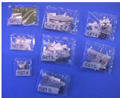
Sample sets sent to Ljubljana for neutron irradiation in JSI TRIGA reactor
